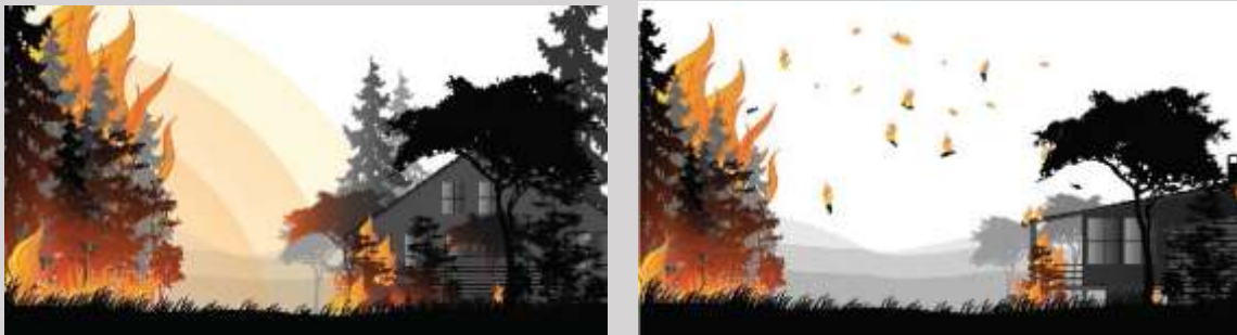
Figure 9: Common sources of home ignition. Burning vegetation can cause intense radiation onto homes (along with flame impingement and hot convective gases) (Left). Firebrand / ember attack from lofted burning material being carried onto homes and causing them to ignite (Right).
